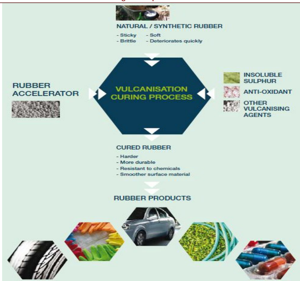
Exhibit 11: Illustration of chemical additives used in making rubber products
